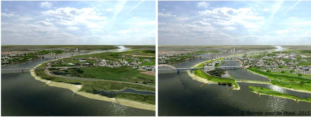
Example of river widening measures at Lent/Nijmegen, Netherlands. Dyke relocations at Lent, right: current situation (after relocation) (programme "Room for the River", project "Room for the Waal" http://www.ruimtevoordewaal.nl )
